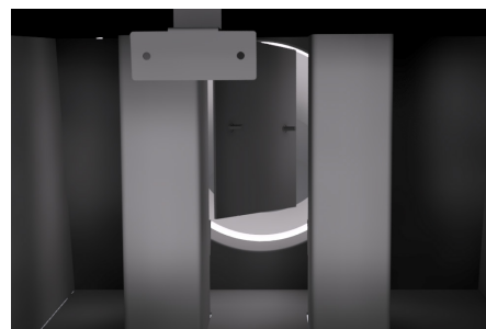
The smoke baffle rests on two channels; slide it forwards, tilt and lower it to remove it.
