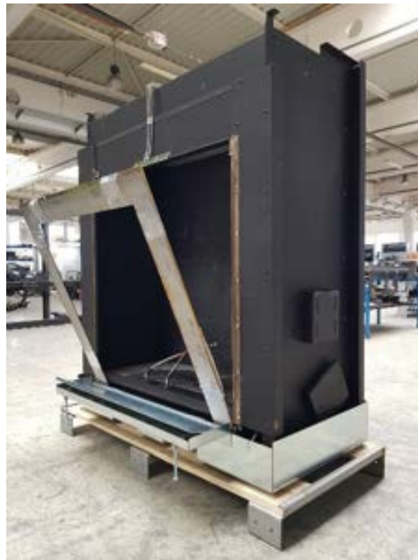
Door fully open: the tilting plate must be slanted as in the picture
