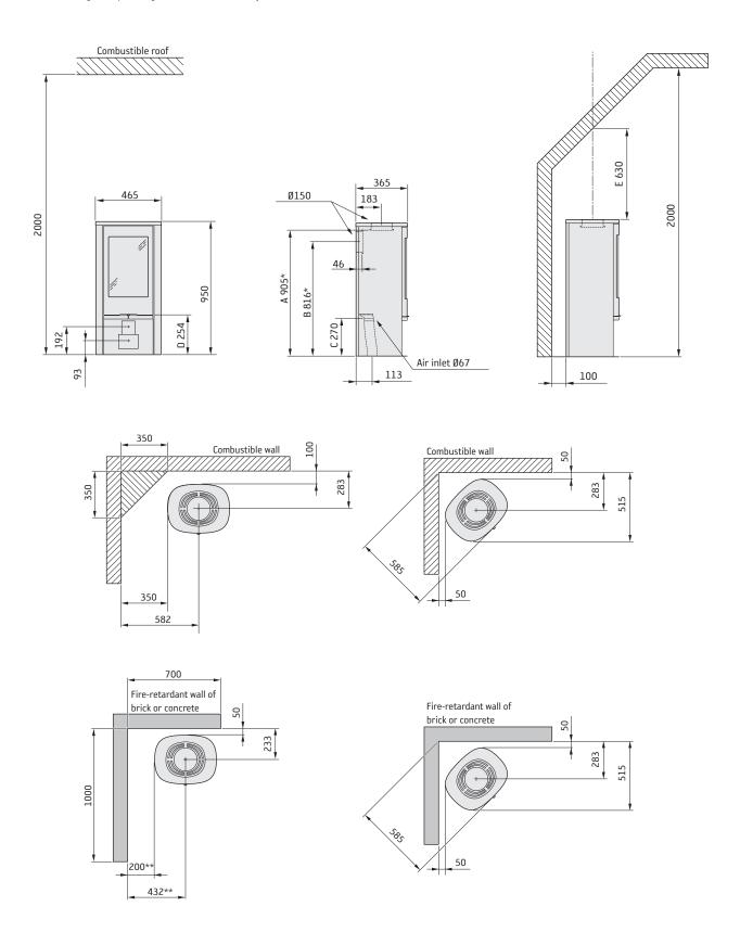
If the stove is placed on a floor protector hearth plate made of glass for example (accessory option), the height from the floor will be increased by the thickness of the hearth plate; for a freestanding glass hearth plate this will be 10 mm.
